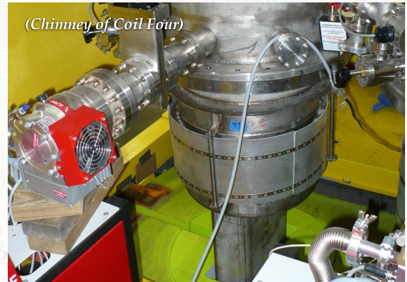
(Temporary Patch of Solenoid Leak)
